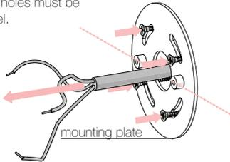
!! Use appropriate screws and plugs for the material you are fixing it to. !!
